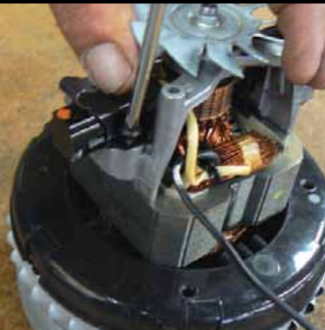
Place the replacement brush onto the comm-end bracket, making certain the positioning post on the bottom of the nylon is placed in the appropriate slot on the bracket. Reassemble the clamp and install screws.
