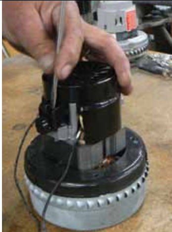
Use a regular screwdriver to pry loose the fan cover.
